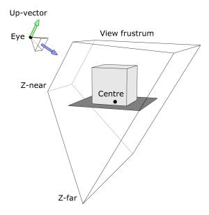
The location of the camera is specified by Eye vector. The look at point is defined by the centre, finally the local y-direction is controlled by the Up-vector.
