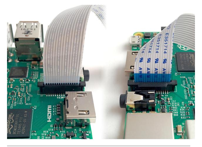
**Note:** If you also need to have a SenseHAT installed, make sure that you stick the cable through the slot on the SenseHAT first. Otherwise it will be difficult to install the PiCamera after you install SenseHAT.
