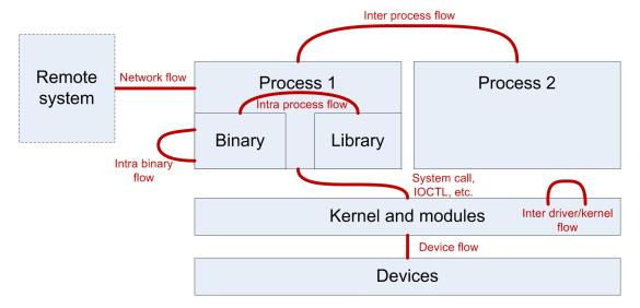
Netzob can handle multiple kinds of input data. Hence, you can analyze network traffic, IPC communications, files structures, etc.
