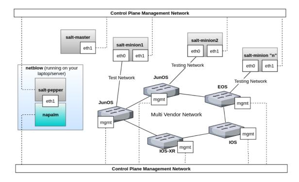
A general idea of how netblow is designed to perform network failures stress tests in the control plane is illustrated below.
