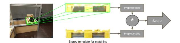
The 3D world coordinates of the corners of the pallet front are calculated. Then the corners are reprojected into the image using the simple relation y = Cx, where x is the world coordinate, C the camera matrix and y the image coordinate. See the wikipage for more background about the camera parameters https://en.wikipedia.org/wiki/Camera\_matrix.
