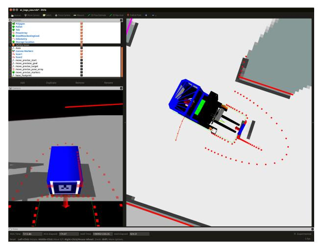
The visualization of the safety fields turns red when some obstacle (red arrow) is in the stop field (red rectangle). This completly stops the truck from moving in that direction.
