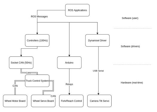
The servo has a position interface and the drive motor a velocity interface.
