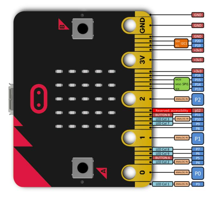
Those pins are available as attributes on the microbit module:microbit.pin0 - microbit.pin20.
