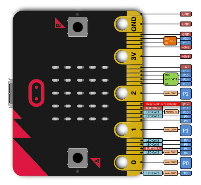
This table summarises the pins available, their types and what they are internally connected to. The pins are available as attributes on the microbit module: microbit.pin0 - microbit.pin20.
