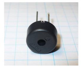
We're going to use an active piezo buzzer for output. To attach one to your BBC micro:bit you should attach crocodile clips to pin 0 and GND (as shown below).
