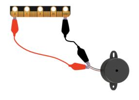
Note: Do not attempt this with an active Piezo buzzer - such buzzers are only able to play a single tone.
