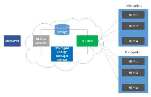
MEMCloud consists of five main components that include storage, RESTful Services, IoT Unit, Microgrid Energy Manager (MEM) and MEMWeb.
