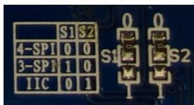
For this display, the two 0 Ohm (jumper) resistors have been connected to “0” and the table shows that “0 0” is 4-wire SPI. That is the type of connection that is currently supported by the SPI mode of this library.
