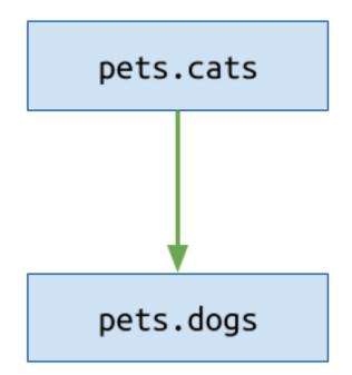
Note the direction of the arrow, which we'll use throughout: the arrow points from the imported module into the importing module.
