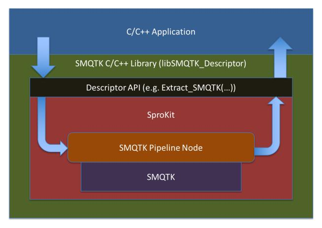
Fig. 1.1: Block Diagramm of the SMQTK/C++ Bridge
