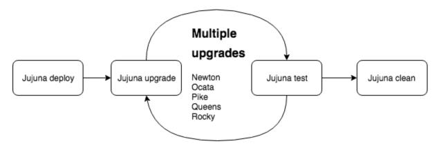
We use Jujuna for three main purposes at HUNT Cloud, all to test desired deployments and service upgrades of OpenStack. We utilize a dedicated stack of test hardware, with very similar configuration to our production site. We deploy the OpenStack Juju bundle with all the applications that we have in production, although at a smaller scale.
