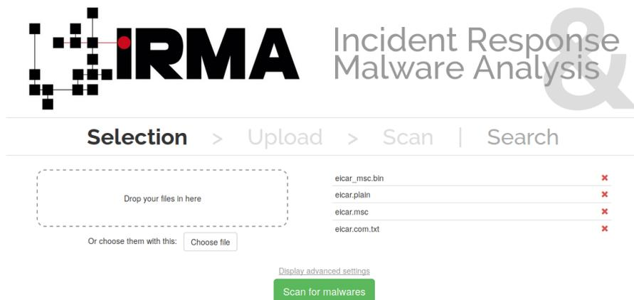
In the scan parameters you can choose if the scans will be forced, meaning that the files are unconditionally scanned, even if there is a cached result. You can choose too which probes will be launched.
