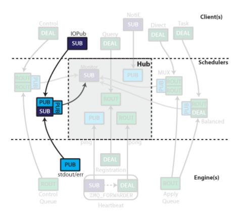
Fig. 2.6: stdout/err are published via a  ${\tt PUB/SUB}$  MonitoredQueue
