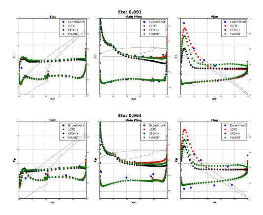
Case 2b, Solar mesh (50M cells),  $Mach=0.175, Re=15e6, \alpha=7^\circ$
