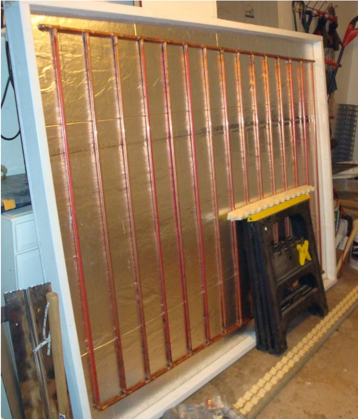
Now, copper is a really good conductor of heat, but with this arrangement, we're only getting the sunlight that directly hits the copper pipe. The reflective insulation might help a little, but we want to catch as much direct sunlight as possible and transfer it to the copper pipes. Most of the designs I've seen use aluminum fins, wrapped around the copper pipe, to transfer this heat, and I think it's an excellent idea.
