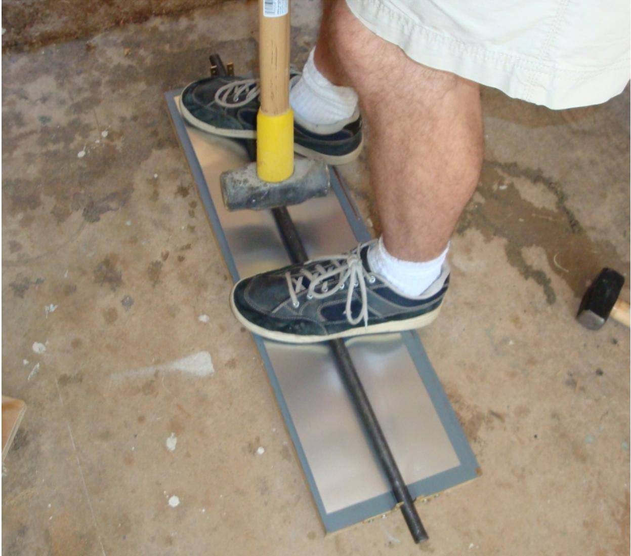
Aluminum flashing is pretty springy, so they don't keep the shape very well, but it's a pretty good start at having the wrap-around profile I'm looking for. In order to mitigate possible galvanic corrosion between the aluminum and copper, I painted the inside grooves black using high-temperature barbecue paint. It doesn't need to be black, but I was planning to use this paint on the rest of the fins anyway.
