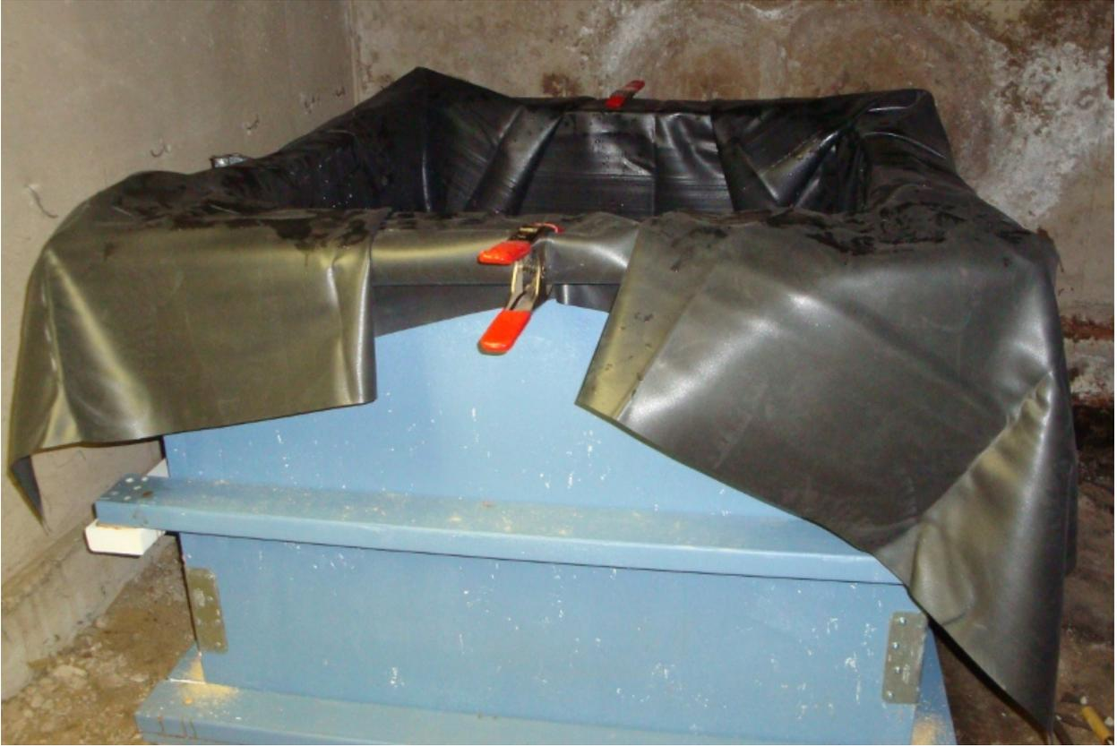
It seemed to help to fill up the tank part of the way before the final attachment of the liner; this made sure that the liner was pressed all the way down into the corners.
