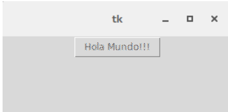
Figura 14.17: Usando disabledforeground sin darle ningun valor
