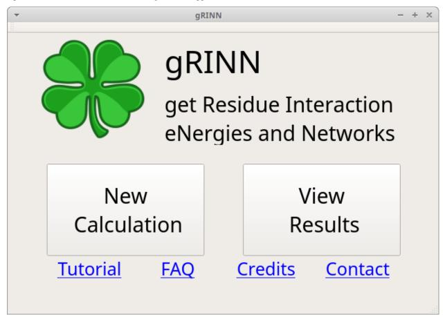
This is the main window of gRINN. The links at the bottom direct the user to respective sections of this website. gRINN offers two interfaces: *New Calculation* and *View Results*.
