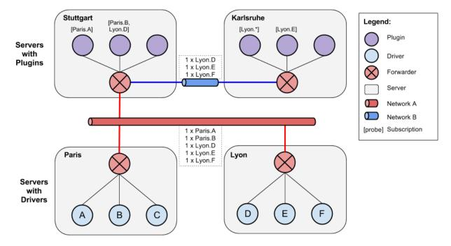
Using the forwarder is optional, and the plugins can be configured to subscribe directly to the drivers. Direct subscribing without using the forwarder is recommanded if the drivers and the plugins are running on the same machine.
