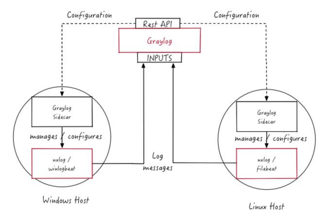
The log collector configurations are centrally managed through the Graylog web interface. Periodically, the Sidecar daemon will fetch all relevant configurations for the target, using the *REST API*. On its first run, or when a configuration change has been detected, Sidecar will *generate* (render) relevant backend configuration files. Then it will start, or restart, those reconfigured log collectors.
