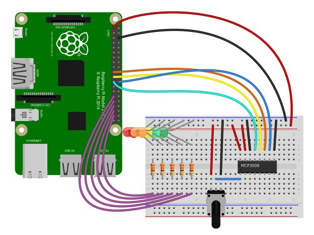
Continually print the value of a potentiometer (values between 0 and 1) connected to a *MCP3008* analog to digital converter:
