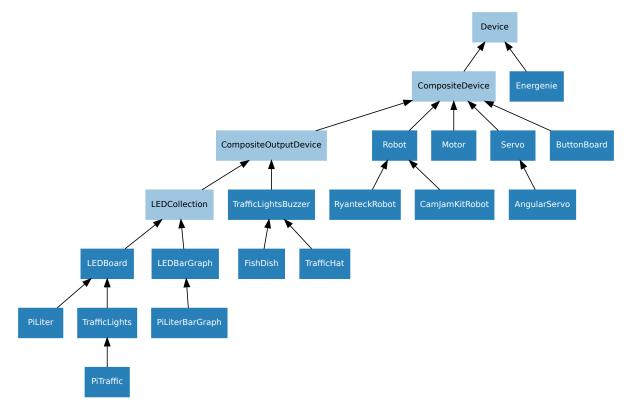
For composite devices, the following chart shows which devices are composed of which other devices:
