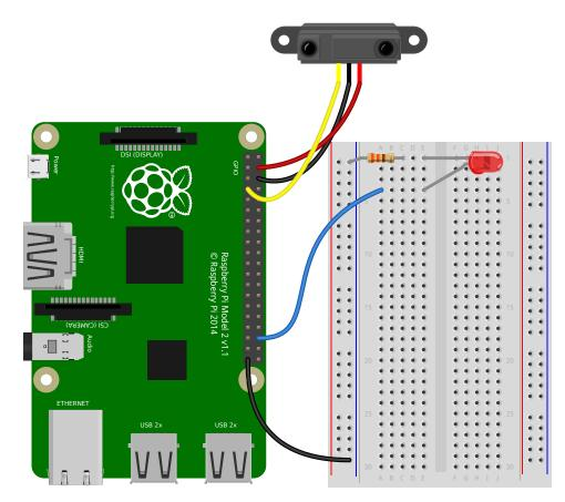
Light an LED when a MotionSensor detects motion:
