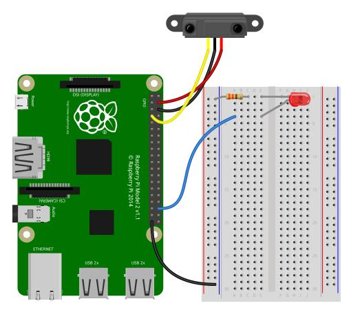
Light an LED when a MotionSensor detects motion:
