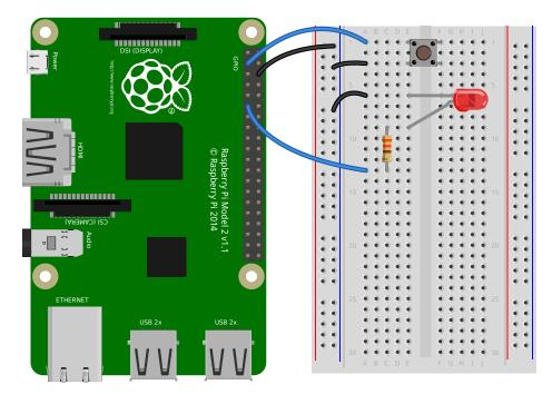
Turn on an LED when a Button is pressed:
