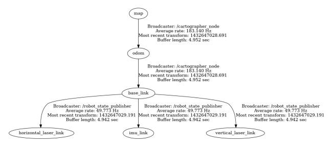
Transforms from all incoming sensor data frames to the *configured tracking\_frame* and *published\_frame* must be available. Typically, these are published periodically by a *robot\_state\_publisher* or a *static\_transform\_publisher*.
