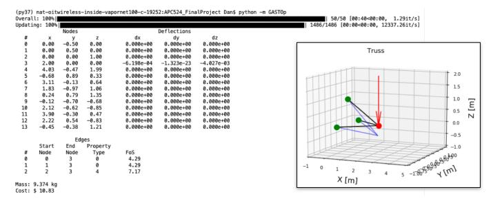
Here the fixed nodes are shown in green, the loads are shown in red, and the truss is shown in black. The blue lines show how the truss deforms under the load magnified by a factor of 50 to be visible. The evolution of the optimization algorithm is shown here:
