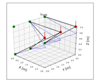
Here the fixed nodes are shown in green, the loads are shown in red, and the truss is shown in black. The blue lines show how the truss deforms under the load magnified by a factor of 50 to be visible.
