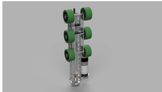
Fig. 53: 11115 Gluten Free, Rover Ruckus, Actobotics lead screw used for hang
