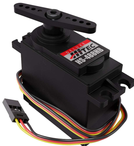
Fig. 8: A common servo, HS488-HB from Hitec
