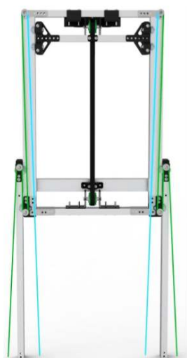
Fig. 55: Example rigging setup from team 7236 Recharged Green. This setup utilizes a continuous stringing setup for the first stage and a cascaded belt-driven second stage.
