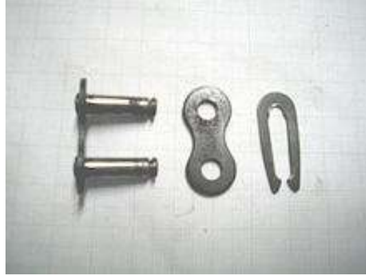
Fig. 24: The removable master link is shown on the right.
