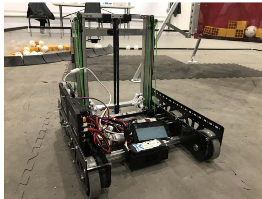
Fig. 50: 7236 Recharged Green, Rover Ruckus, custom box tube linear elevator
