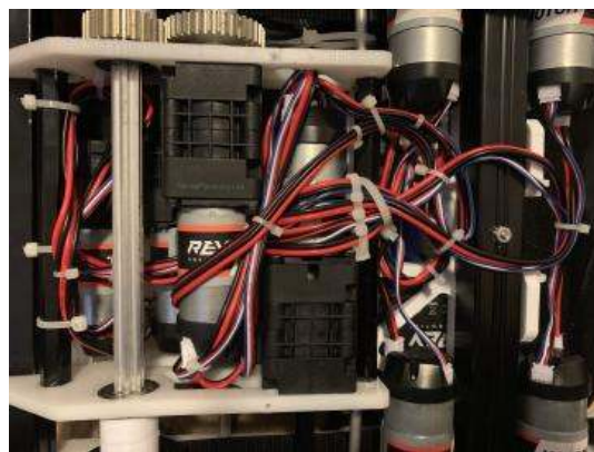
Fig. 2: Good example of wiring by 731 Wannabee Strange, Rover Ruckus
