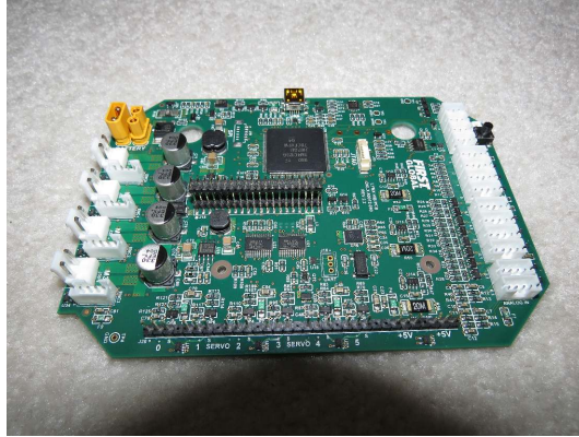
Fig. 4: A Lynx board that was removed from its case
