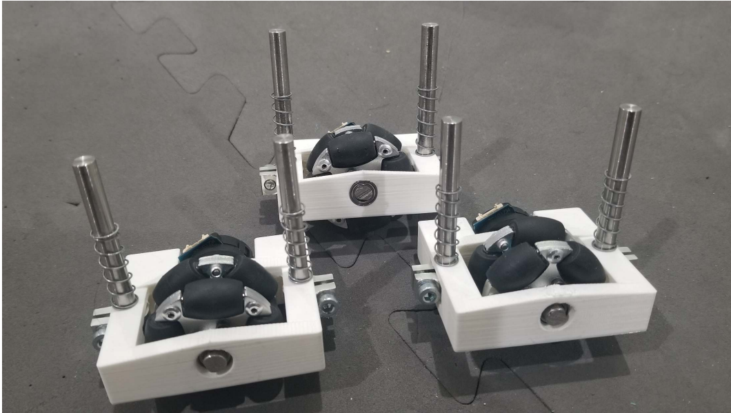
Fig. 106: FTC 18172's vertical springing
