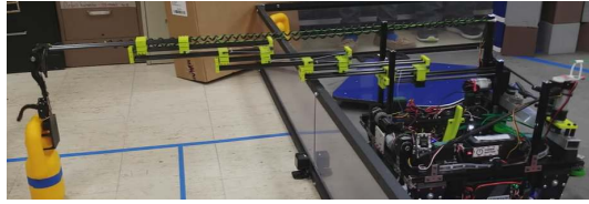
Fig. 47: 5975 Cybots, Relic Recovery, round linear bearings and carbon fiber tubes with 3D printed mounts
