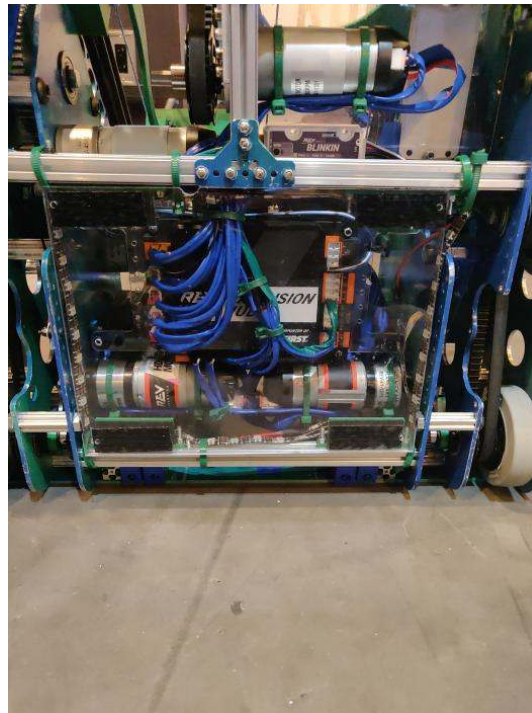
Fig. 3: Good example of wiring by 8417 'Lectric Legends
