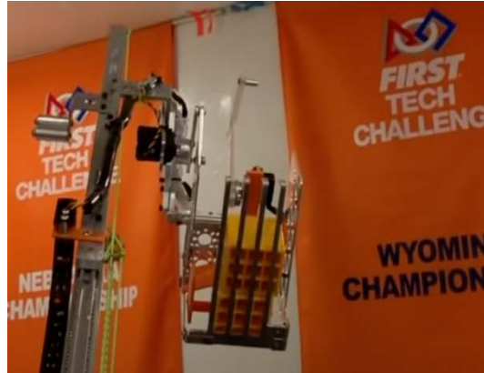
Fig. 97: 6929 Data Force, Rover Ruckus, Grate transfer deposit. Forks are visible on the bottom, which go between forks on the intake bucket.
