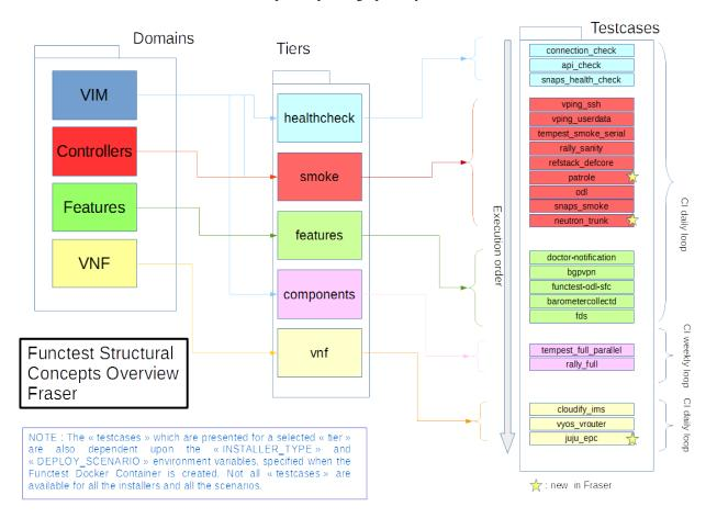
Some of the test cases are developed by Functest team members, whereas others are integrated from upstream communities or other OPNFV projects. For example, Tempest is the OpenStack integration test suite and Functest is in charge of the selection, integration and automation of those tests that fit suitably to OPNFV.
