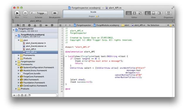
The ForgeModule subproject is used to contain the code and resources for your plugin, and the ForgeInspector outerproject is the sandbox you can run and test your plugin in before packaging it up to send to Trigger.io.
