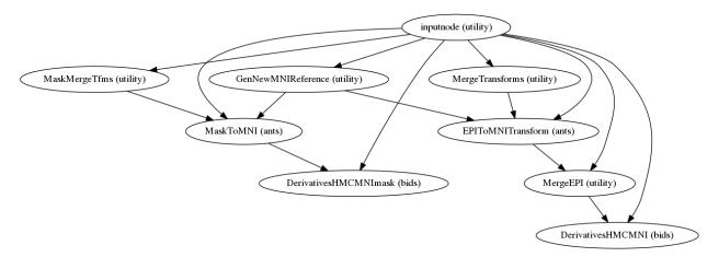
The EPIMNITransformation sub-workflow uses the transform from  $ref\_epi\_t1\_registration$  and a T1-to-MNI transform from  $t1w\_preprocessing$  to map the EPI image to standardized MNI space. It also maps the t1w-based mask to MNI space.
