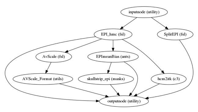
The EPI\_HMC sub-workflow collects BIDS-formatted EPI files, performs head motion correction, and skullstripping. FSL MCFLIRT is used to estimate motion transformations and ANTs is used to apply them using Lanczos interpolation. Nilearn is used to perform skullstripping of the mean EPI image.
