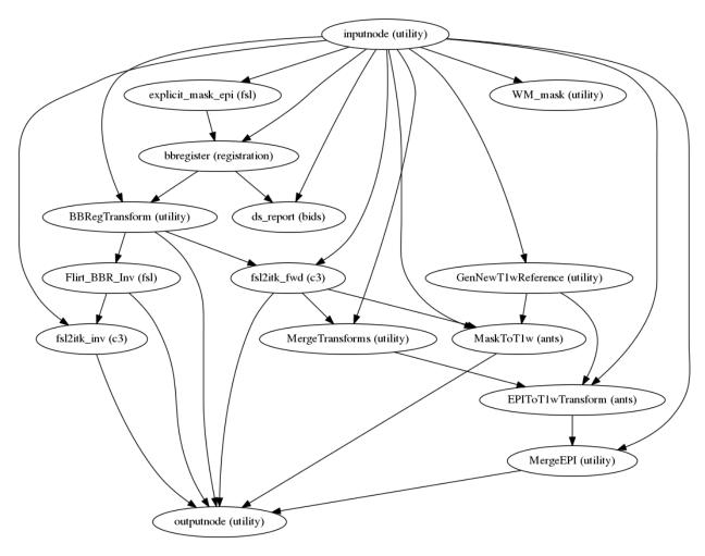
The  $ref_epi_t1_registration$  sub-workflow uses FSL FLIRT with the BBR cost function to find the transform that maps the EPI space into the T1-space.
