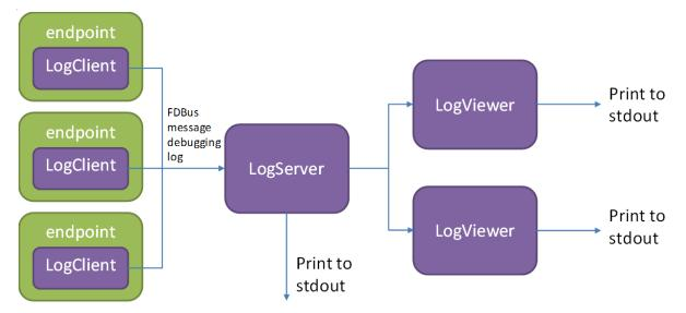
Like the normal server, the log server runs up and registers with the name server, which broadcasts the LogClient in each endpoint. Later, when the endpoint sends an FDBus message, it will also send a copy to the log server through
