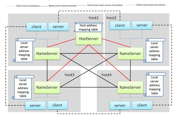
In the above figure, a star connection is established between the name server and the host server, and the name server and the name server are connected one by one to form a network. In this system, the main tasks of the name server and host server are:
