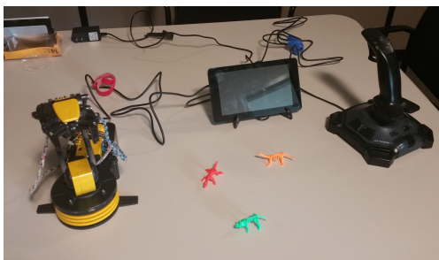
Fig. 1.18: RasPi, joystick, and RoboArm connected
