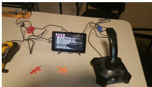
Fig. 1.19: RasPi starting up after power is applied.
