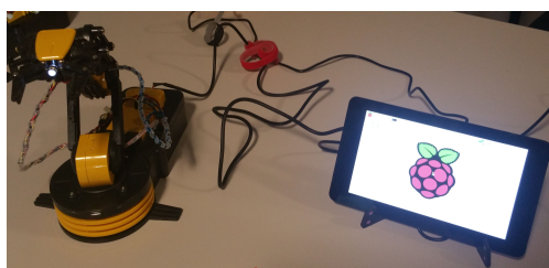
Fig. 1.20: The RoboArm LED is ON indicating the EPICS IOC has started.
