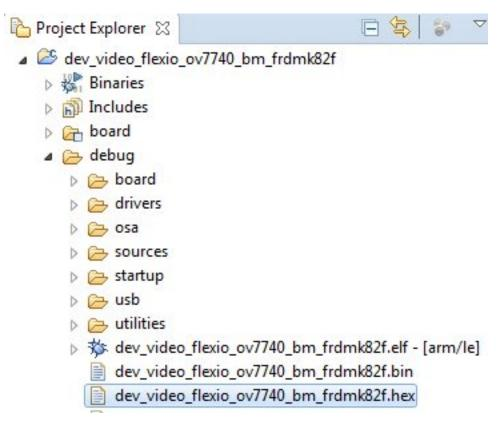
6. The **dev\_video\_flexio\_ov7740\_bm\_frdmk82f.hex** file is the firmware demo uploadable in the FRDM-K82F, it is used in *Quick Start Guide*
