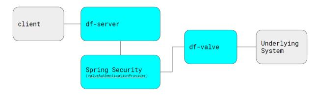
As can be seen in the diagram above, **df-server** leverages Spring security to handle authentication. This is done via the ValveAuthenticationProvider. Spring Security is configured to use this authentication provider which calls the **authenticate()** method of IValve. The authenticate method is responsible for executing the necessary elements to authenticate with the underlying system.
