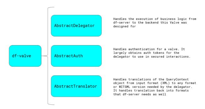
As seen in the diagram above, each component of the valve is defined as an abstract class that can then be implemented by the valve implementation.
