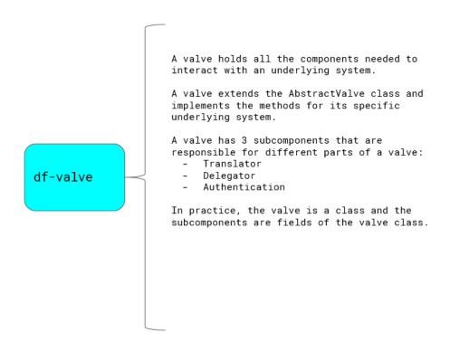
As seen in the image above, the valve is an encapsulation of all the elements required to communicate with an underlying system.
