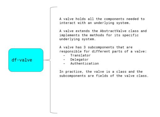
As seen in the image above, the valve is an encapsulation of all the elements required to communicate with an underlying system.
