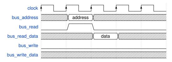
Peripherals connected to the bus must present valid data one clock cycle after the *bus\_read* signal is asserted. This allow using FIFO blocks with *read-ahead* option disabled, which is more performant.
