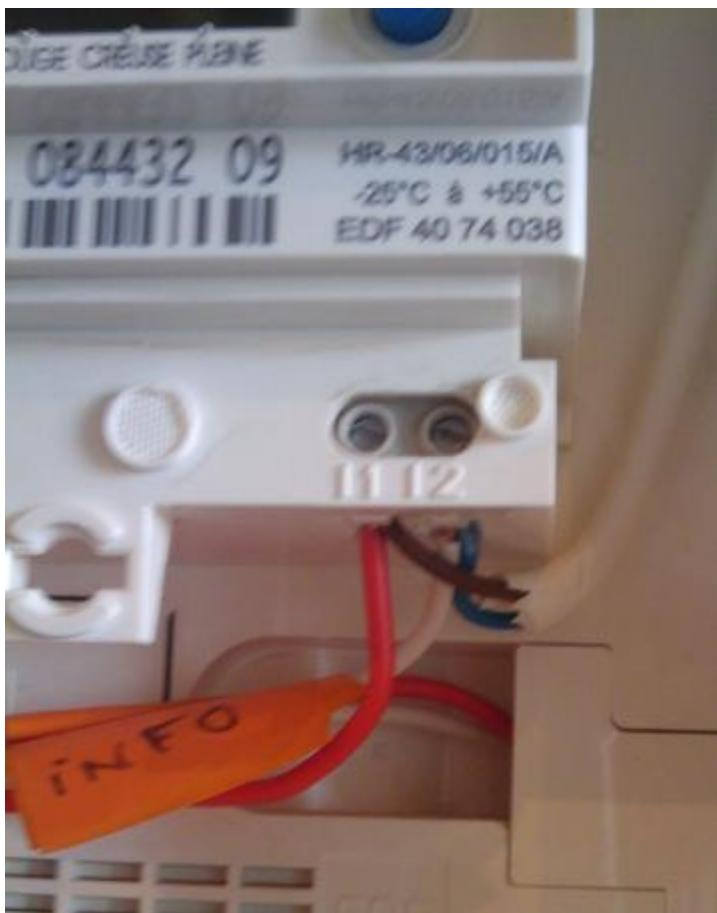
Here is the Usb teleinfo modem : on the left, the usb plug, on the right, the 2 wires that are plugged on I1 and I2:
