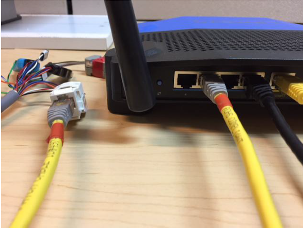
Fig. 5: Figure 5 Connect an ethernet cable between the ethernet connector and a router
