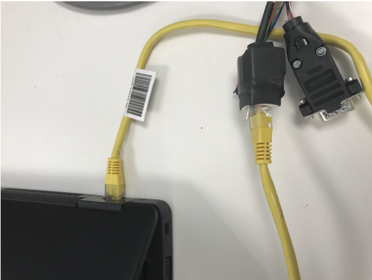
Fig. 4: Figure 4: Connect an ethernet cable between the ethernet connector and a computer
