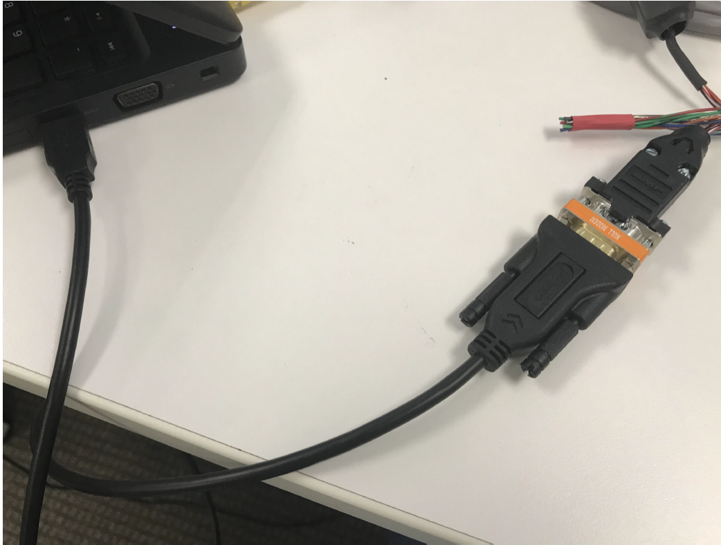
Fig. 3: Figure 3: Connect the serial usb to computer
