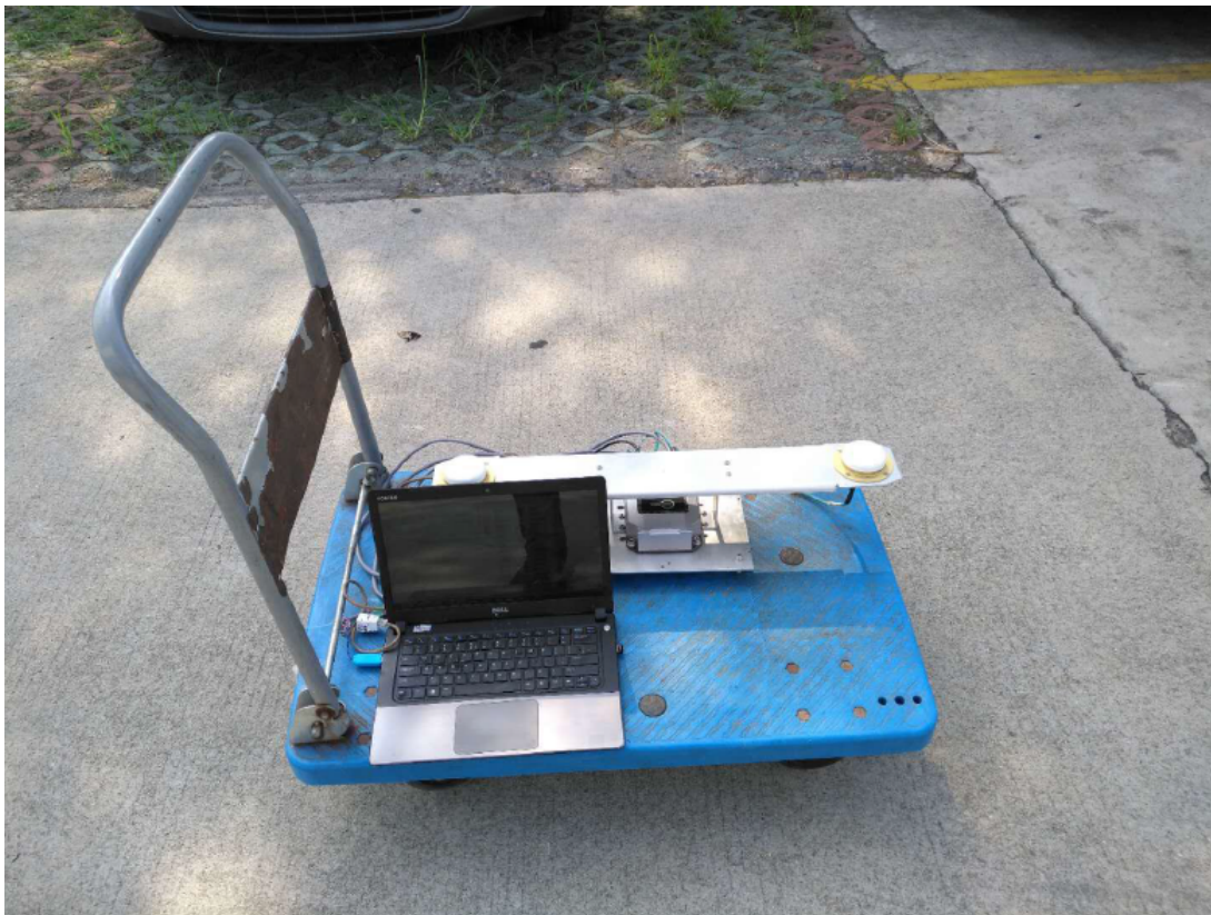
Fig. 3: Figure 5: Laptop computer jamming the GNSS
