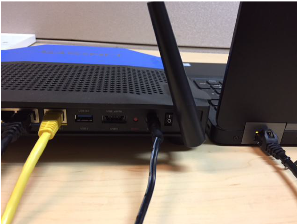
Fig. 6: Figure 6 Connect an ethernet cable between the router and a computer
