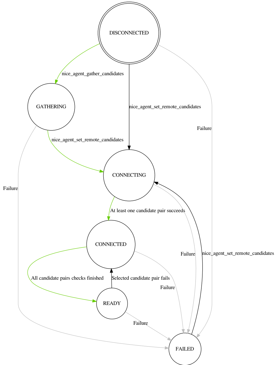
Fig. 1: libnice state transition diagram for NiceComponentState
