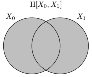
Next, the conditional entropy of  $X_0$  conditioned on  $X_1$ ,  $HX_0|X_1$ , is displayed. It consists of the area contained in the  $X_0$  circle but not contained in  $X_1$  circle.
