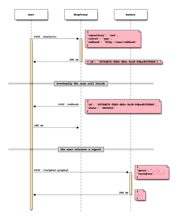
The sequence diagram above shows the typical usage workflow.
