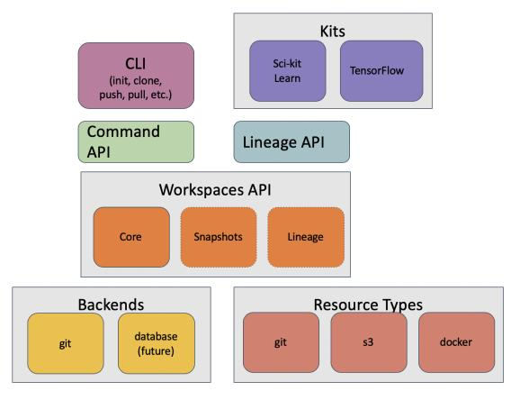
The core of the system is the Workspaces API, which is located in dataworkspaces/workspace.py. This API provides a base Workspace classes for the workspace and a base Resource class for resources. There are also several mixin classes which define extensions to the basic functionality. See *Core Workspace and Resource API* for details.
