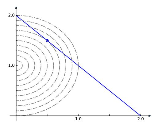
We return to the textbook model and set the solver to one that can handle quadratic objectives such as cplex. We then add the linear constraint that the sum of our x and y reactions, that we set to FBA and NH4t, must equal 2.
