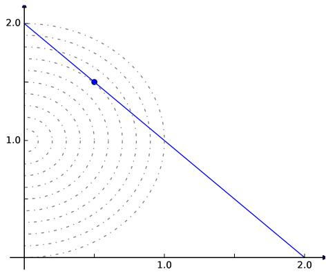
QP solvers in cobrapy will combine linear and quadratic coefficients. The linear portion will be obtained from the same objective\_coefficient attribute used with LP's.
