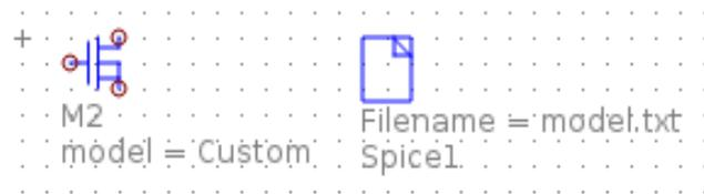
The advantage of using an external library file over the previous methods is that you can download the needed model or library from the web and use it directly in your design without needing to manually copy every parameter to a *model component*. This method is similar to that found in commercial simulation programs.
