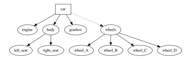
The diagram declares that car consists of engine, gearbox, body and a set of wheels, completely ommiting the properties of each object.
