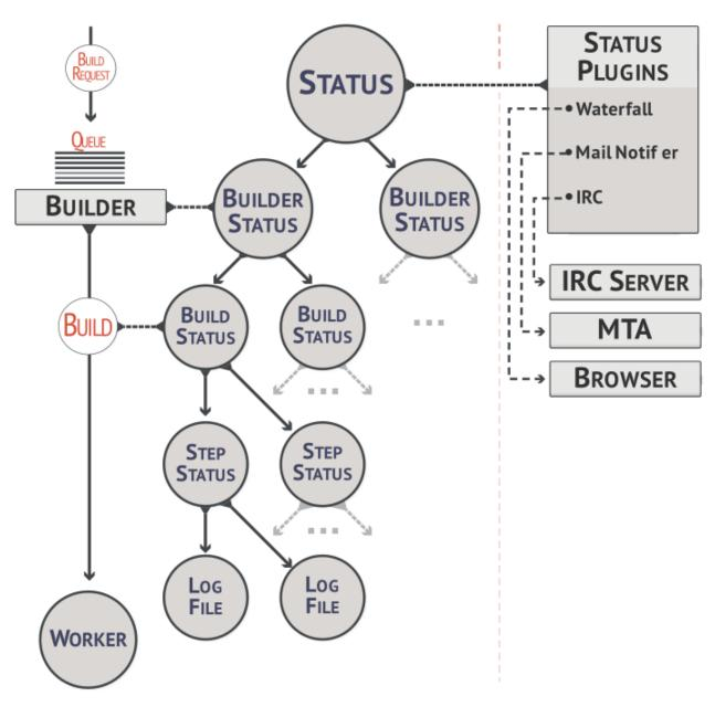
The configuration file controls which status plugins are active. Each status plugin gets a reference to the top-level Status object. From there they can request information on each Builder, Build, Step, and LogFile. This query-on-demand interface is used by the html.Waterfall plugin to create the main status page each time a web browser hits the main URL.
