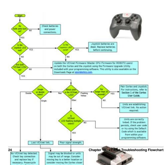
If the issue is still present after following this guide, update both the Cortex and Joystick with the most recent version of the VEXnet Firmware (Master CPU Firmware for ROBOTC users). If this does not resolve the problem, try using a different set of VEXnet keys. If you need further assistance you can post a question on the VEX Forum (https: //vexforum.com) or contact VEX Technical Support by phone at +1-903-453-0802 or email support@vexrobotics.com.
