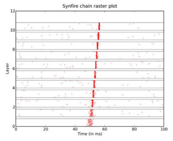
The simulation of 1000 neurons in 10 layers, each all-to-all connected to the next, using integrate and fire neurons with synaptic noise for 100ms of simulated time took 1 second to run with a timestep of 0.1ms on a 2.4GHz Intel Xeon dual-core processor. The next image is of the state space, figure 3:
