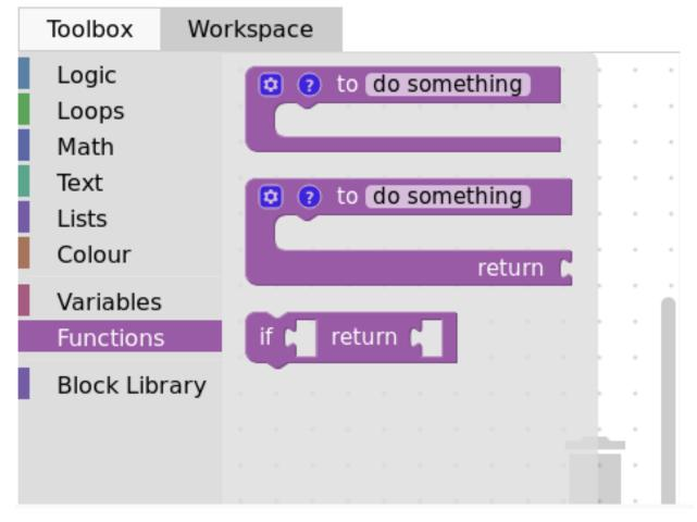
Now, configure the function. The wheel icons allow us to add parameters. Simply name your parameter (x by default), then connect the block into the right space, like so :
