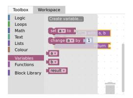
Finally, select the corresponding block and plug it into the "return" spot. Here is our basic workspace done, with the preview :
