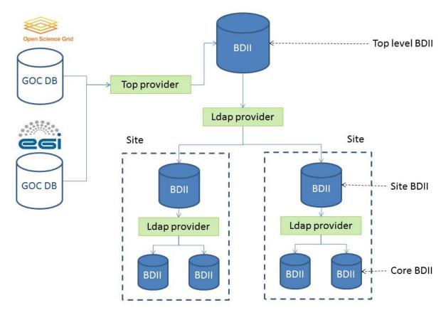
The BDIIs are populated with information by running information providers. These are scripts which obtain information, format it as LDIF and print the result to standard out. These information providers can also be used to query other BDIIs which is how the hierarchy is built. The order in which these information providers are run is random.
