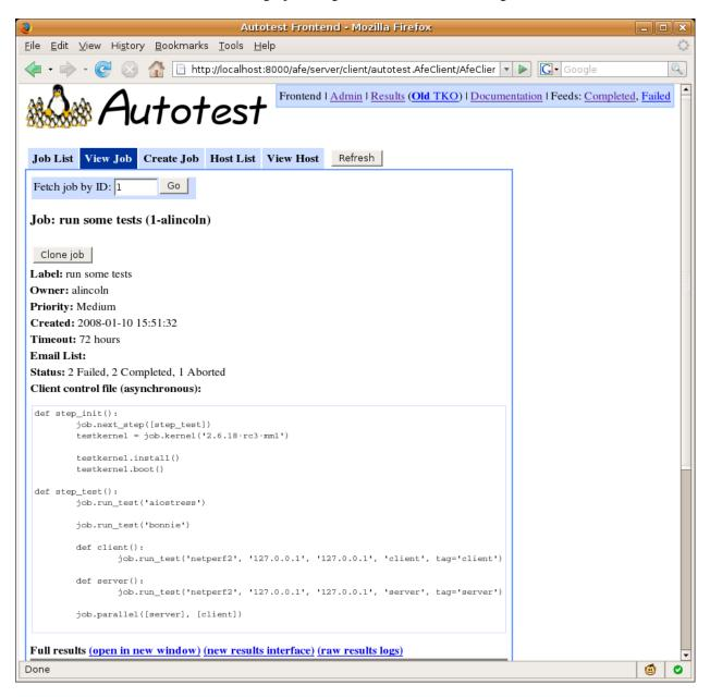
The box at the top allows you to manually fetch a job by ID. The page displays basic info about the job, an "Abort Job" button if the job has not completed, and a "Clone Job" button to create a new job modeled after the current job. Clone job will present three options:
