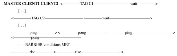
Note that once the last client has responded to pong the barrier is implicitly deemed satisifed, they have all acknowledged their presence. If we fail to send any of the rlse messages the barrier is still a success, the failed host has effectively broken 'right at the beginning' of the post barrier execution window.
